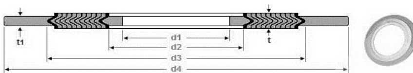
Dimensions of Spiral Wound Gaskets to suit API 605 Flange
