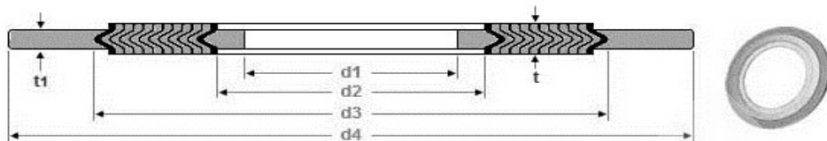
Dimensions of Spiral Wound Gaskets as per BS 3381 to suit BS 1560 Flange
